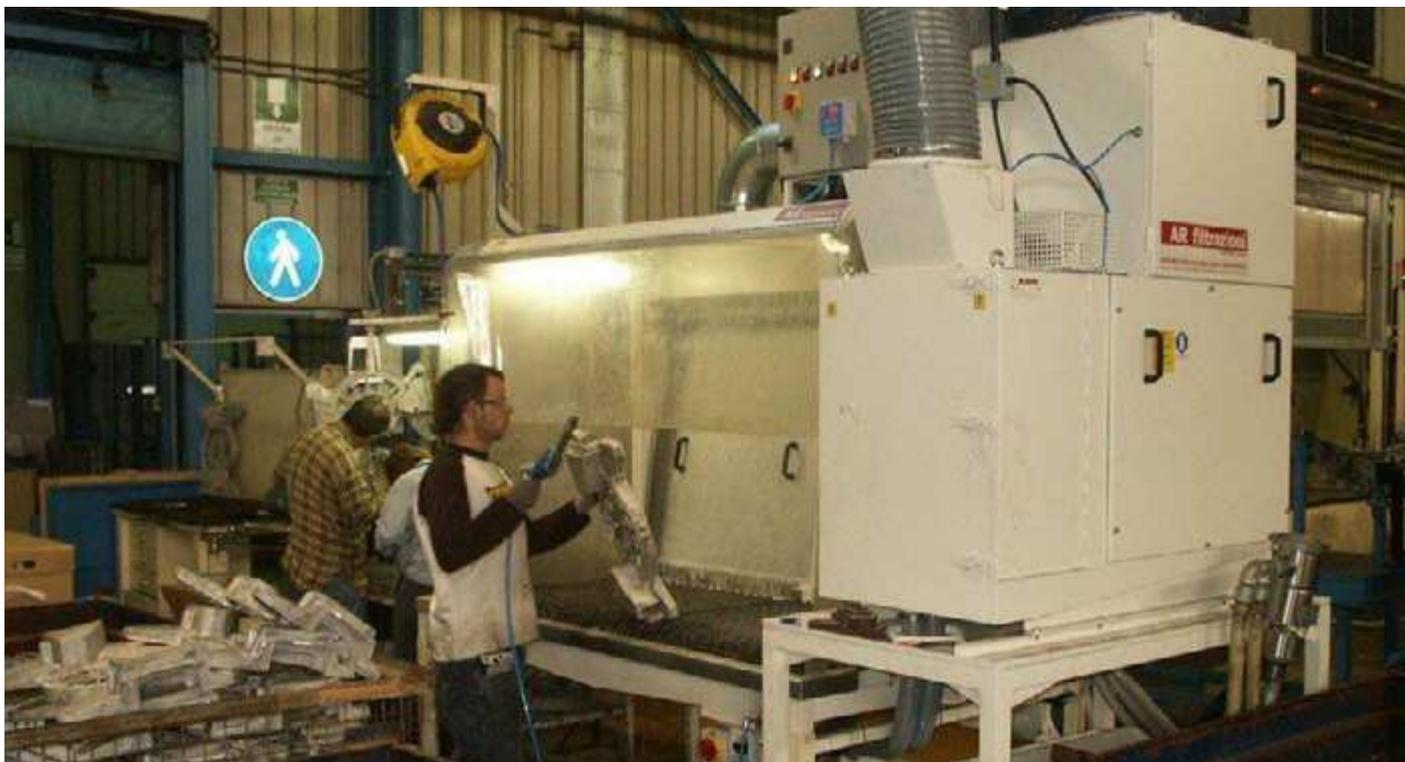
HYDROFILTER E HIDRODESK PARA LA REBABA MANUAL EN SECO DEL MAGNESIO
